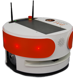
Fig. 4. PMB2: the modular mobile base used in TIAGo
