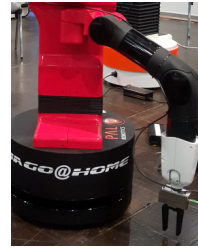
Fig. 11. Integration of a third party end-effector
