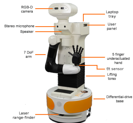
Fig. 2. TIAGo main specs
