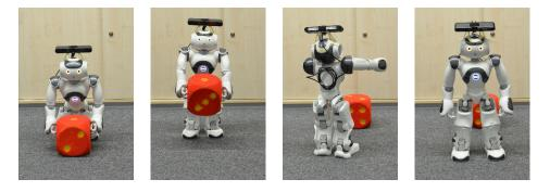
Fig. 10. Picking up: The pick up action includes the tracking of the object locally, positioning relative to the object, executing the grabbing, performing a  $180^{\circ}$  turn, dropping the object, and rotating back  $180^{\circ}$ .
