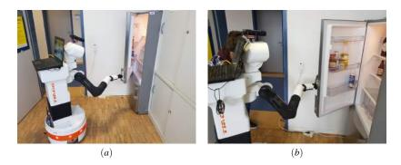
**Figure 1** TIAGo first detected the handle of the fridge and opened it (a) After taking the beer it is closed again (b).
