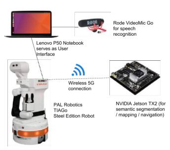
Figure 4 Hardware Architecture
