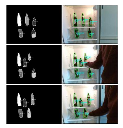
**Figure 7** Example labels using the trained model on 5 beer brands. The labels are 'Koblenzer', 'Erdinger', 'Bitburger', 'Ginger' and 'Karlskrone'. On the left you see the networks output and on the right the post processed result.
