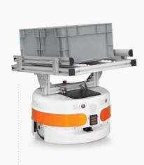
**TIAGo® Static Roller** Able to transfer the load by fixed conveyors and transport it anywhere.
