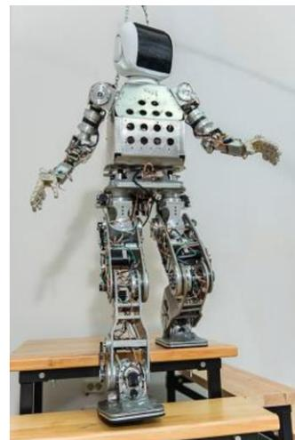
Figure 1. Anthropomorphic robot AR-600E, source <http://npo-at.com/products/ar-600e/>
